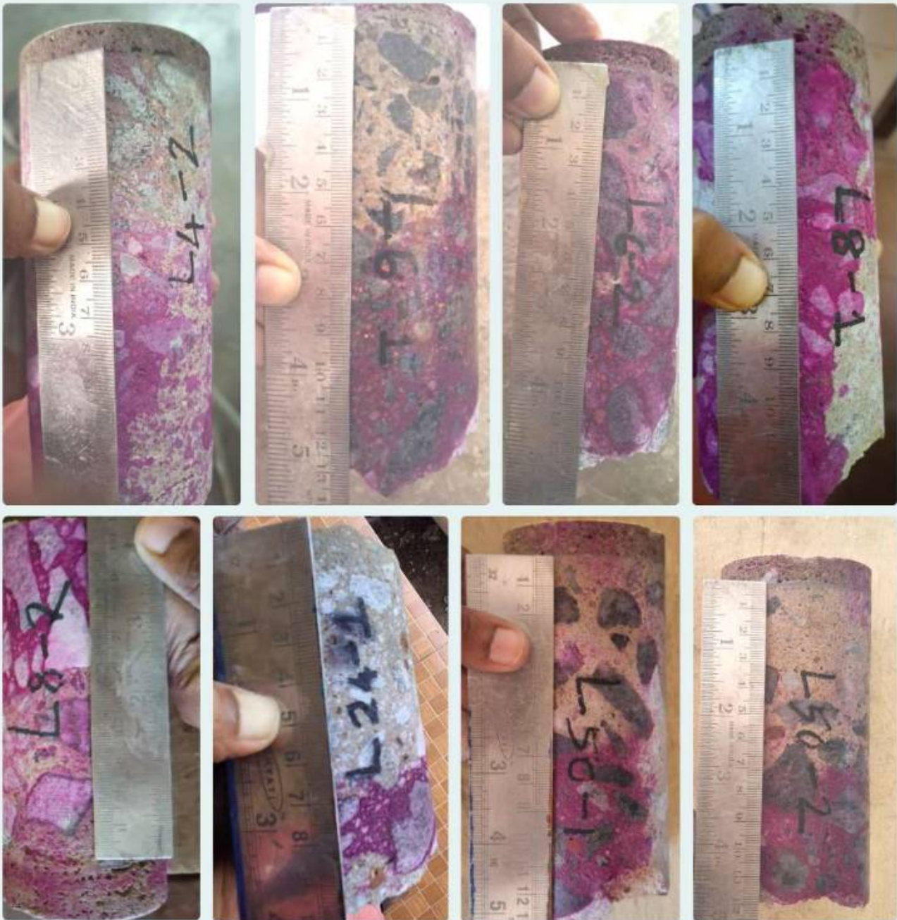
Carbonation test on concrete cores
