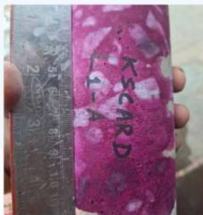
Carbonation test on extracted concrete core specimen
