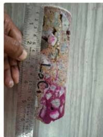
Carbonation test on extracted core specimens
