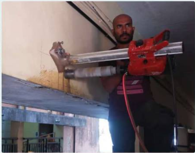
Extraction of concrete core specimen from Beam
