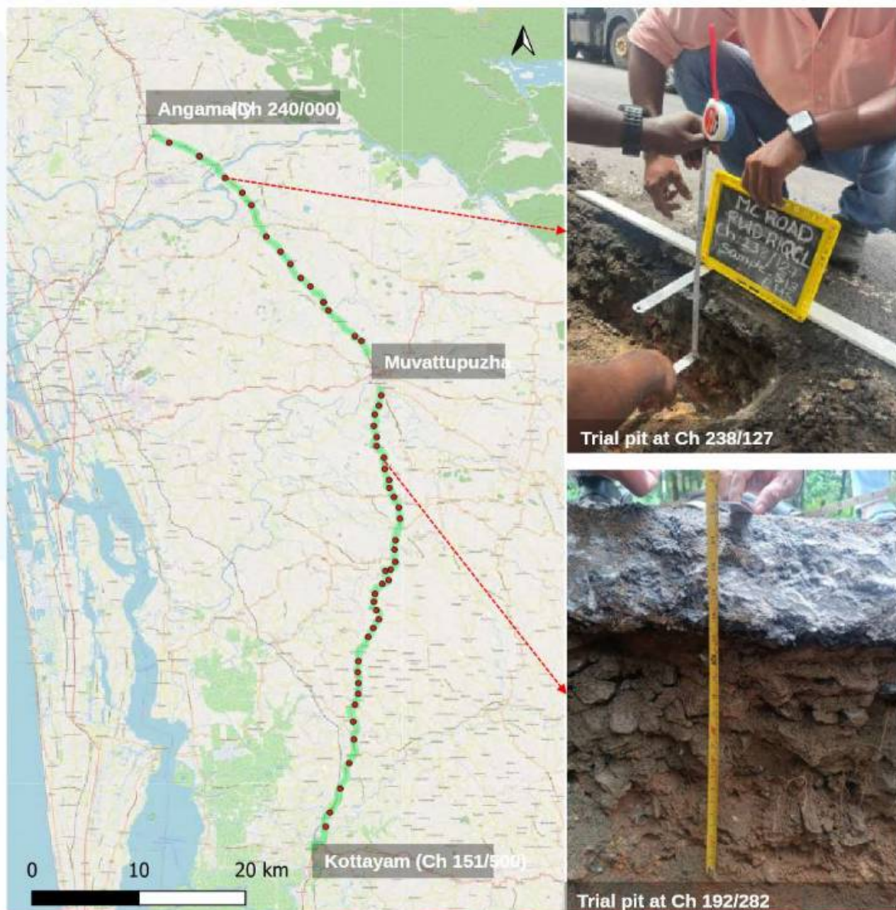
Trial pit survey locations done by PWD, RIQCL, Ernakulam
