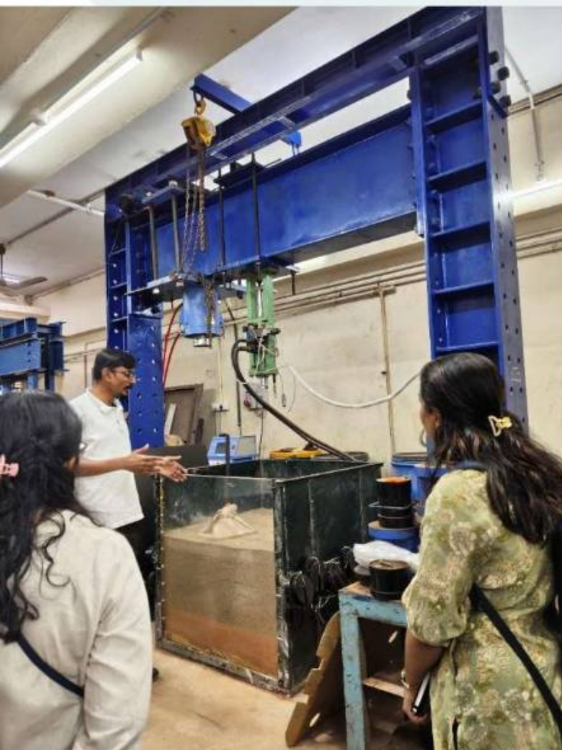
Cyclic plate load test setup
