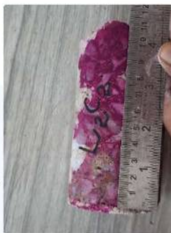
Carbonation test on extracted core specimens
